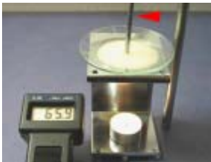
Experimental arrangement for measuring the temperature development during cooling with Water Jel dressings.
